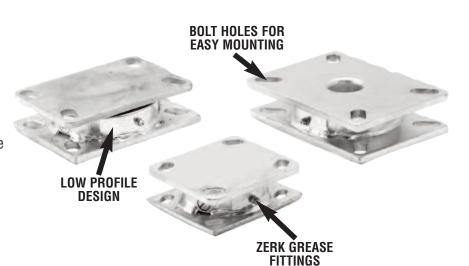
"Forged Steel" Construction • Plates are AISI 1045 steel one-piece forging precision machined and through-hardened. Bearing mounted on precision machined raceway.
