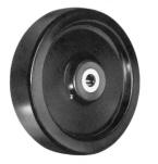
Wheels are molded of heavy macerated or chopped canvas, impregnated with phenolic resin and accurately formed in close fitting molds under high pressure and temperature.
