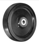
Wheels are molded of heavy macerated or chopped canvas, impregnated with phenolic resin and accurately formed in close fitting molds under high pressure and temperature.
