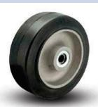
Cushion rubber treads are vulcanized to die cast aluminum core. The soft rubber tread affords a cushion effect to the load and excellent floor protection. These wheels are highly shock absorbing and provide quiet operation, while dampening vibration.
