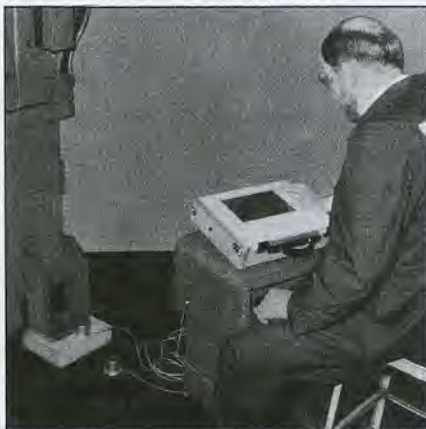
ENGINEER MEASURES VIBRATIONS
