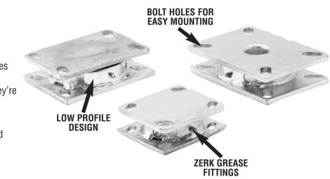
"Forged Steel" Construction • Plates are AISI 1045 steel one-piece forging precision machined and through-hardened. Bearing mounted on precision machined raceway.
