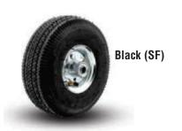
Full Pneumatic (SF) Recommended for the greatest possible protection to both loads and floors. If you transport fragile materials or parts, or if you move delicate instruments over rough floors, you should consider a pneumatic tire. Full pneumatics cushion the load on air, just like an automobile. They must be properly inflated as indicated in wheel table. Can be filled with urethane foam to make them deflation proof, but foam has no effect on capacity. Suitable for extended service.
