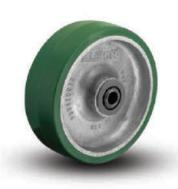
Composed of a polyurethane elastomer, open cast or injection molded, on clean, close tolerance cores. Polyurethane tread is chemically bonded to aluminum core. High capacity polyurethane protects floors, is non-marking and delivers quieter operation than standard metal wheels. PA wheels feature **cast** aluminum core. PD wheels feature **die cast** aluminum cores.
