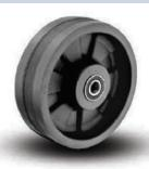
Similar to NG wheels, but with the added benefit of two rubber treads on the wheel edges to reduce noise and improve traction even under heavy loads. Not recommended for towing applications above 3mph. Temperature range is -40° F to +180° F.
