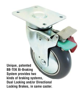
**Green Pedal Directional Lock:** Locks the swivel in one direction but wheel remains free for tracking straight line.
