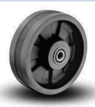
Similar to NG wheels, but with the added benefit of two rubber treads on the wheel edges to reduce noise and improve traction even under heavy loads. Not recommended for towing applications above 3mph. Temperature range is -40° F to +180° F.
