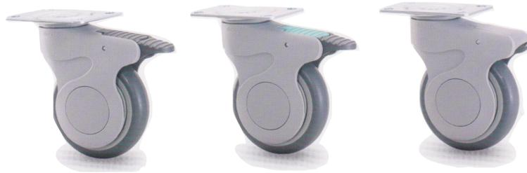
**P Top Plate Fitting** Glass fiber reinforced Nylon 6 for body and brake pedals. Precision ball bearings at swivel head and wheel axle. Non-marking, elastic thermoplastic polyurethane treads.
