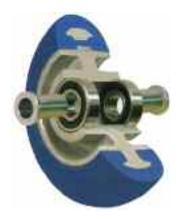
Donut Tread Urethane Wheels are ergonomically designed with rollability in mind. These premium polyurethane wheels are standard with crowned treads, sealed precision ball bearings and top had reducing bushings for optimum rollability. These wheels will perform well in both manual and power-towed material handling applications. They are available in four different tread durometers (hardness) and color coded for easy identification.
