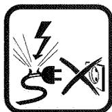
Check the machine, cable and plug each time the machine is used. Only have damage repaired by a qualified professional.
