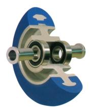
Donut Tread Urethane Wheels are ergonomically designed with rollability in mind. These premium polyurethane wheels are standard with crowned treads, sealed precision ball bearings and top hats reducing bushings for optimum rollability. These wheels will perform well in both manual and power-towed material handling applications. They are available in four different tread durometers (hardness) and color coded for easy identification.
