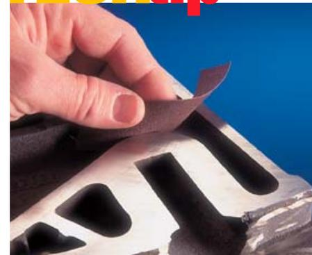
Use light machine oil with cloth rolls as a lubricant for finer finishes and quicker cut.
