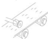
Generating pulses from idler roll with RPG
