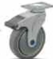
Our Directional Lock casters are designed to lock the swivel but not the wheel allowing you to steer your equipment. The directional lock feature is designed to break free under heavier load when the unit is traversing a corner only to lock back into position when the unit resumes a straight course.
